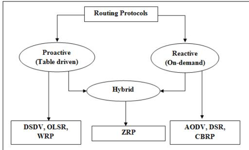
**Figure 4: MANETs Routing Protocols**
