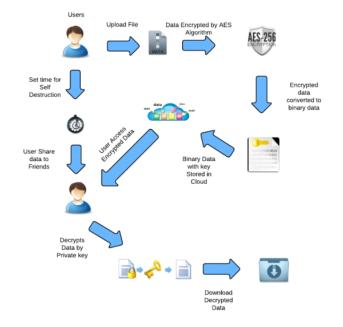
Fig 1. System Architecture
