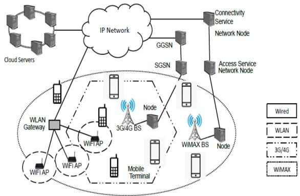
Fig. 1. Mobile cloud computing uses everywhere mobile phones connect to cloud servers via various network interfaces such as WiFi, cellular network, and WiMax
