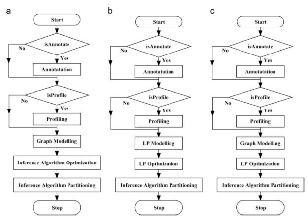
Fig. 6. A flowchart of Optimal partitioning algorithms for MCC (a) Graph-based, (b) LP based and (c) hybrid based
