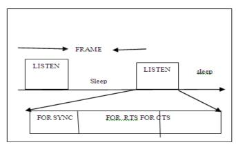
Figure 1: Low Duty Cycle Operation of S-MAC [3]
