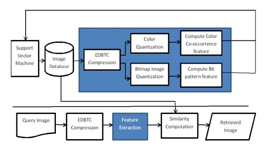
Fig.1 Schematic diagram of proposed image retrieval framework
