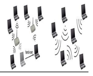
(a) An infrastructured network with two base stations. (b)A mobile ad-hoc networks.
