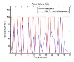
Figure 4.6: Percentage of Packet delivery ratio for proposed algorithm
