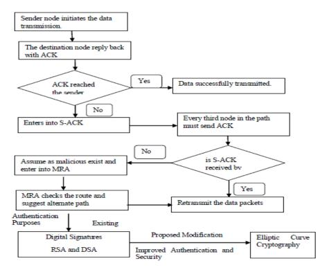
Fig-1 System Flow Diagram
