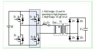
Fig.1: Reconfigured LLC topology from full bridge to half bridge
