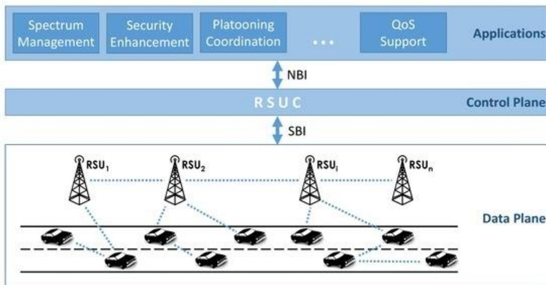
Figure 1. Architecture diagram of DA Platoon System
