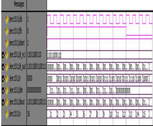
Figure 5: Simulated Waveform for (15, 11, 1) BCH Encoder
