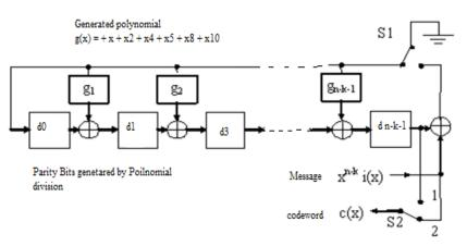
Figure: 1. Encoder circuit for a (n, k) BCH code
