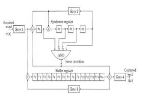
Figure 9 Decoder block diagram for (15, 11, 1) BCH decoder
