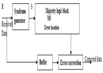
Figure 8 BCH Decoder design
