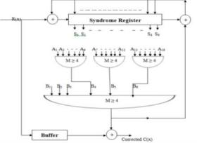
Figure 11. Decoder block diagram for (15, 5, 3) BCH decoder
