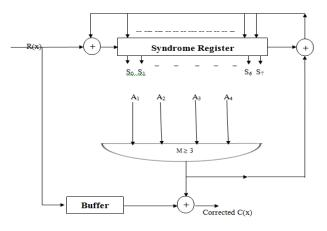
Figure 10 Decoder block diagram for (15, 7, 2) BCH decoder
