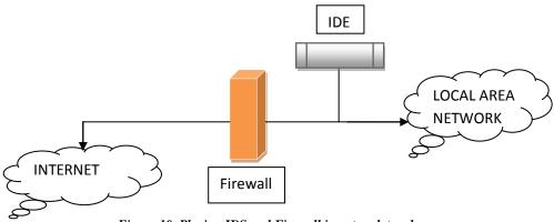
Figure 10. Placing IDS and Firewall in network topology
