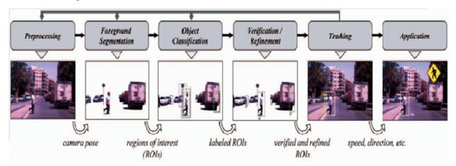
Fig1. Architecture for an On-board Pedestrian detection system
