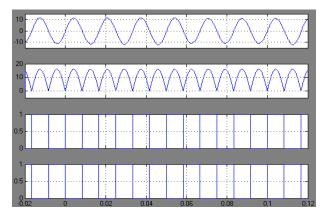
Fig 6. .Simulation results for full-bridge inverter of the five-level inverter.(a) Output current of the full-bridge inverter *io* . (b) Input current of the full bridge inverter *id* . (c) Driver signal of S4 . (d) Driver signal of S5 .
