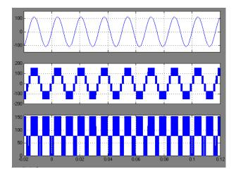
Fig.7. Simulation results of the five-level inverter. (a) Utility voltage. (b) Output voltage of the full-bridge inverter. (c) Output voltage of the dual buck converter.
