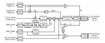
Fig.4. Control block diagram of five-level inverter.
