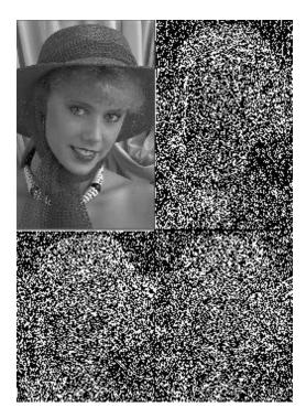
Fig.2: Wavelet transformed image
