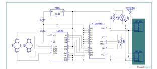
Fig 3 circuit diagram of car module
