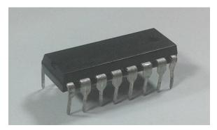
Fig 1 ASK hybrid transmitter
