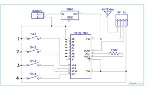
Fig 4 circuit diagram of control module
