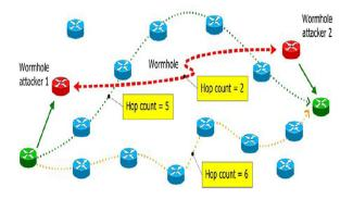
Fig.1: Wormhole Attack in wireless networks
