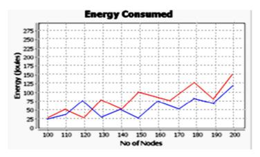
Fig.8: Energy vs No of nodes Red line- Multiple base stations with always Blue line- Multiple base stations during detection
