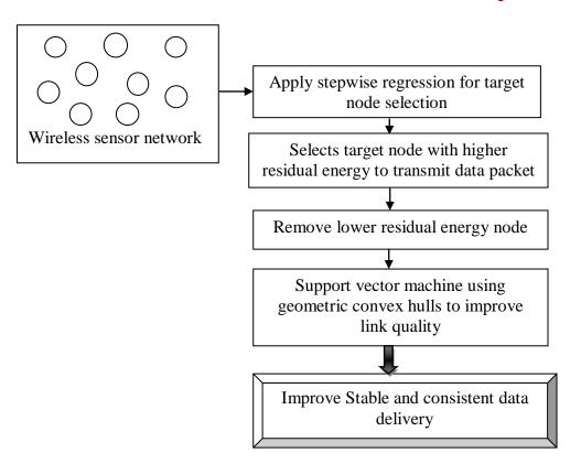
Figure 1 Architecture Diagram of Stepwise Regression based Support Vector Machine technique
