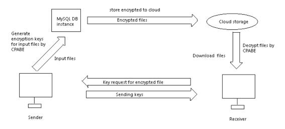
Fig 1. Encryption and Decryption Architecture
