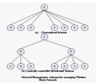
Fig. 6. Network management schemes (a) conventional (b) Centrally controlled
